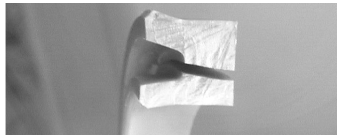
Fig. 1: Seal damage section view
