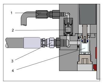
Fig. 4: Auto-bleeder integrated in Safety Catcher series K/TA
