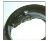
Fig. 4: Seal damage, section view
