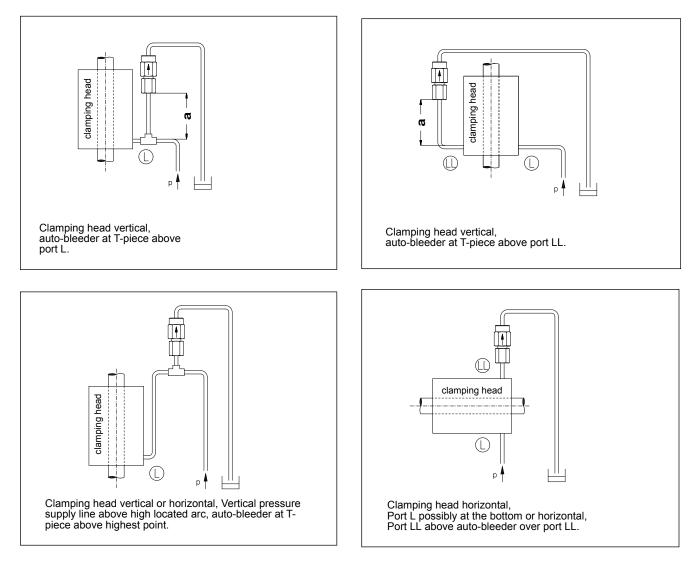
Clamping heads with 2 pressure connections (KB series) need a second auto-bleeder for port K in the same way described above for port L.
