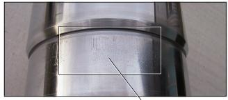
Fig. 4: Damages to sealing surface
