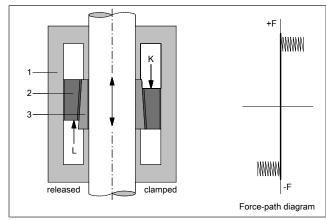
Fig. 1: Functional basics of a Locking Unit
