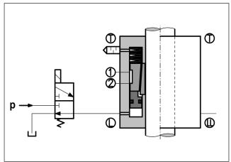
Fig. 2: Actuation of Locking Unit
