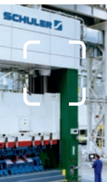
Hydraulic press Safety Catcher as DGUV-approved restraint device
