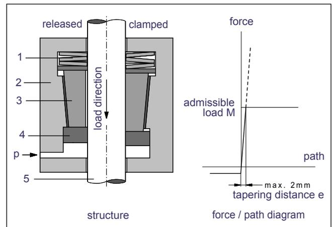
Fig. 1: Functional principle
